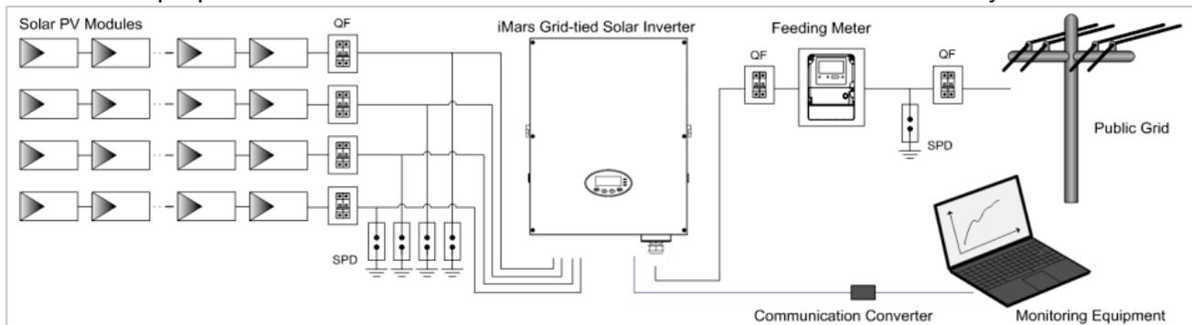
Figure 4.14 Block diagram of the grid-tied solar system
