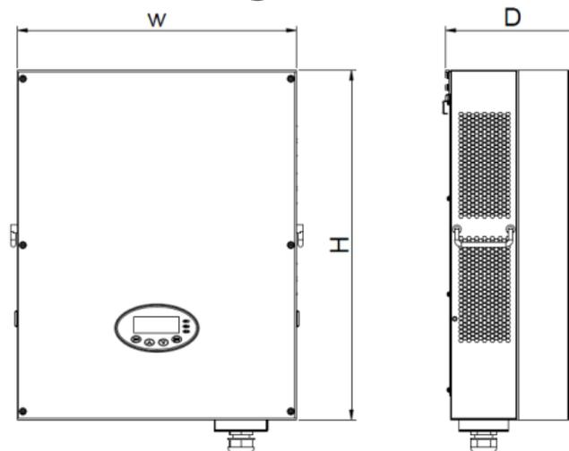
Figure 2.7 Inverter dimensions
