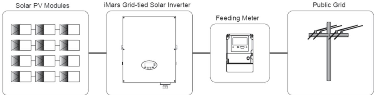
Figure 2.1 Application of iMars grid-tied solar inverters
