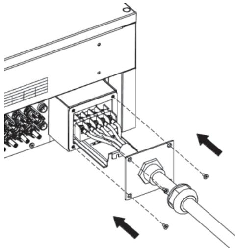
Figure 4.22 Fix the waterproof cover of junction box
