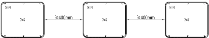
Fig 4.5 Size requirements for side-by-side installation
