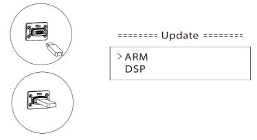
4) Press "Up" and "Down" to select ARM or DSP. Then long press "Down", and select the correct update file to confirm the update. ARM and DSP shall be updated one by one.
