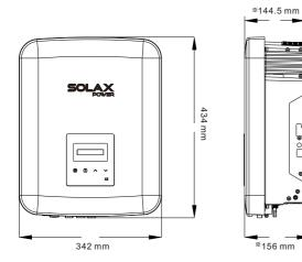
X3-MIC G2 Size(3 kW, 4 kW, 5 kW, 6 kW): 342 mm\*434 mm\*144.5 mm X3-MIC G2 Size(8 kW, 10 kW, 12 kW, 15 kW): 342 mm\*434 mm\*156 mm
