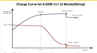
Phase 1: The Max. charge current is 2.0A, and the charge voltage is gradually risen up to 57.6V;
